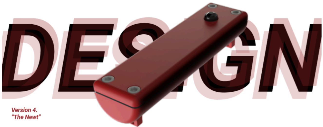
Figure D: Physical Form Factor of Baton V2a, or "The Newt," which is for optimal fixturing, especially a flat face for attaching the button.
