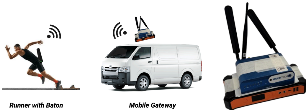
Figure 5 & 6: Mobile Race Gateway. This includes the SIM Card TTN Gateway with the Portable JIYHF P100 Power Station fitted below. This device would be placed in the window of the followers car or stationary along the runner path at a central position.
