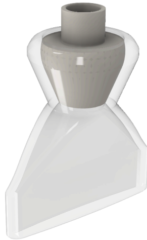
Figure 12. Isometric View of Nozzle Assembly (Nozzle rendered as transparent to show nozzle adapter geometry)
